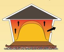
The heat pattern from heaters and radiators shows that much of the heat rises to the ceiling and is lost through windows, leaving the living area of the room as the last area to heat up.
