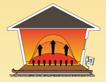
With Warmup Undercarpet Heating the heat rises gently through the room, delivering heat directly to the living area with minimum heat loss.
